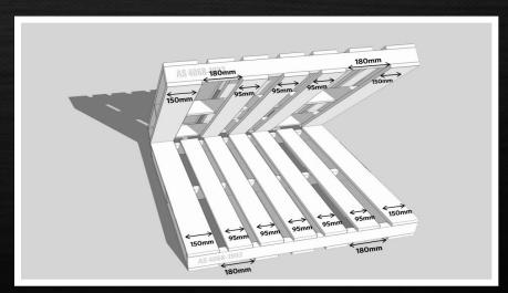
The underside deck of each pallet must be comprised of five boards; two lead boards of 150mm width, and three intermediate boards of 95mm width. Two pallet 'tunnels' of 180mm must also be maintained, between the lead boards and the next intermediate boards
