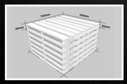
The top deck of each pallet must be comprised of seven or eight boards; two lead boards of 150mm width, and five or six intermediate boards of 95mm width
